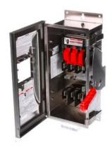
Siemens Low Voltage Circuit Protection Heavy Duty Safety Switches. Type: ENCLOSED, SAFETY SWITCH Std: UL V. Rating: 600V A. Rating: 100A No. Of Poles: 3P F. Rating: 60Hz Action: SINGLE THROW Material: SS Enclosure: TYPE 4X. 2-3 point mounting holes. Insulation: YES O. Cycles: 10000 O. Temperature: (-20F-120F) AMBIENT TEMPERATURE Environmental Conditions: INDUSTRIAL CORROSIVE RESISTANCE
