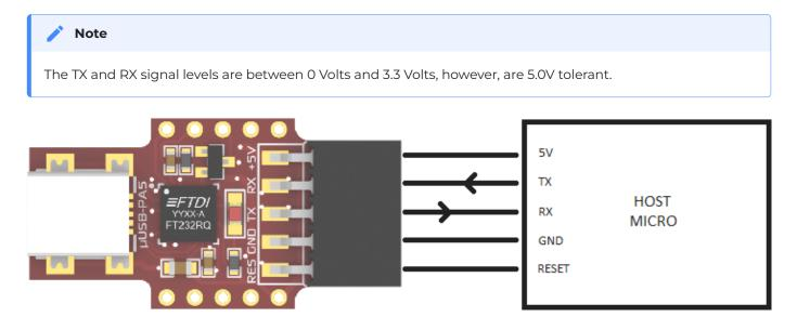
The micro USB is designed to have a compact footprint, and be compatible with prototyping such as plugging it directly into a breadboard when male 2.54mm (0.1") headers are soldered to the row of 5 pins, along each side.
