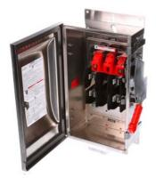
Siemens Low Voltage Circuit Protection Heavy Duty Safety Switches. Type: ENCLOSED, SAFETY SWITCH Std: UL V. Rating: 240V A. Rating: 60A Wattage: 2W No. Of Poles: 2P F. Rating: 60Hz Action: SINGLE THROW Material: SS Enclosure: TYPE 4X. 2-3 point mounting holes. Insulation: YES O. Cycles: 10000 O. Temperature: (-20F-120F) AMBIENT TEMPERATURE Environmental Conditions: INDUSTRIAL CORROSIVE RESISTANCE
