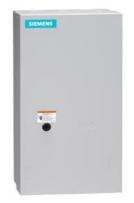
Mechanically held lighting contactor, Contactor amp rating 200A, 0 N.C. / 4 N.O. poles, 110VAC 50HZ/120VAC 60HZ coil, Non-combination type, Enclosure NEMA type 1, Indoor general purpose use
