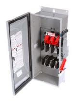
Siemens Low Voltage Circuit Protection Heavy Duty Safety Switches. Type: ENCLOSED, SAFETY SWITCH Std: CSA V. Rating: 240V A. Rating: 30 A Wattage: 3W No. Of Poles: 3P F. Rating: 60Hz Action: SINGLE THROW Material: 304SS Enclosure: TYPE 12. 2-3 point mounting holes. Insulation: YES O. Cycles: 10000 O. Temperature: (-20F-120F) AMBIENT TEMPERATURE Environmental Conditions: INDUSTRIAL
