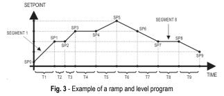
The program created is permanently stored in the controller's memory. It can be modified freely, executed when necessary and repeated as often as necessary.
