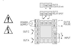
Fig. 1 - Electrical connections of the controller
