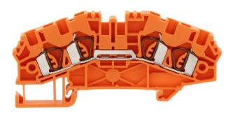
Feed-through terminal, Tension-spring connection, Mounting type: Mounting rail TS 35/7.5, Rated cross-section: 2.5 mm², Width: 5.1 mm, Colour: Orange
