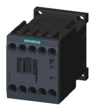
Power contactor, AC-3 9 A, 4 kW / 400 V 1 NC, 42 V AC, 50 / 60 Hz 3-pole, Size S00 screw terminal
