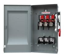
Siemens Low Voltage Circuit Protection Heavy Duty Safety Switches. Type: ENCLOSED, SAFETY SWITCH Std: UL V. Rating: 600V A. Rating: 30 A Wattage: 3W No. Of Poles: 3P F. Rating: 60Hz Action: SINGLE THROW Material: STEEL Enclosure: TYPE 1. 2-3 point mounting holes. O. Cycles: 10000 O. Temperature: (-20F-120F) AMBIENT TEMPERATURE Environmental Conditions: INDOOR
