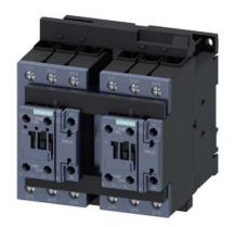
Reversing contactor assembly for 3RA27 AC-3,18,5 kW/400 V,20-33 V AC/DC 3-pole, Size S2 screw terminal electrical and mechanical Interlock 2 NO integrated with voltage tap
