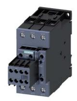
power contactor, AC-3 40 A, 18.5 kW / 400 V 2 NO + 2 NC, 220 V AC 50 Hz / 240 V, 60 Hz, 3-pole, Size S2, screw terminal
