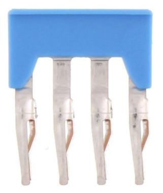
Insulated cross-connector, No. of poles: 4, Mounting type: Plug in, Width: 19.3 mm, Rated cross-section: 2.5 mm<sup>2</sup>, Colour: Blue
