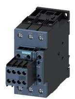
Contactor relay, AC-3 65 A, 30 kW / 400 V 2 NO + 2 NC, 24 V DC with varistor 3-pole, size S2 screw terminals suitable for 2 A PLC outputs
