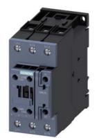
Power contactor, AC-3 65 A, 30 kW / 400 V 1 NO + 1 NC, 24 V AC, 50/60 Hz 3-pole, size S2 screw terminals
