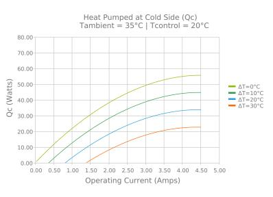
Heat Pumped at Cold Side (Qc) Tambient = 35°C | Tcontrol = 20°C 80.00 70.00 60.00 (Watts) 50.00 ∆T=0°C ΔT=10°C  $\Delta T = 20^{\circ}C$ 40.00  $\Delta T = 30^{\circ}C$ ö 30.00 20.00 10.00 0.00 0.00 5 00 10.00 15.00 20.00 25.00 30.00 35.00 Operating Voltage (Volts)
