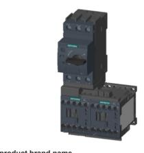
FUSELESS LOAD FEEDER REVERSING OPERATION, 400 V AC, S00 0.45 TO 0.63 A 3 KW, 110/120V AC 50/60 HZ SCREW TERMINAL FOR STANDARD RAIL MOUNTING, TYPE OF COORDINATION 2, IQ = 150 KA (ALSO FULFILLS TYPE OF COORDINATION 1) 1NC (CONTACTOR)
