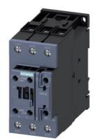
Power contactor, AC-3 65 A, 30 kW / 400 V 1 NO + 1 NC, 48-80 V AC / DC with varistor 3-pole, size S2 screw terminals
