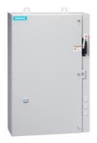
Reversing motor starter, Size 2, Three phase full voltage, Solid-state overload relay, OLR amp range 13-52A, 110V 50Hz / 120V 60Hz coil, Combination type, 60A disconnect switch, Enclosure NEMA type 4/12, Water/dust tight for outdoors
