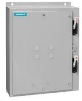
Duplex starter w/o alternator, Size 0, Three phase full voltage, Solid-state overload relay, OLR amp range 3-12A, 240V 50Hz / 277V 60Hz coil, Combination type, Two 10A circuit breakers, Enclosure NEMA type 12, Dust/drip proof for indoors
