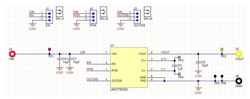
Figure 5. LM2775EVM Schematic
