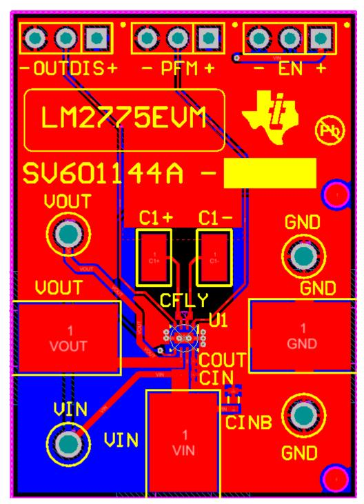
Figure 3. Top Assembly Layer
