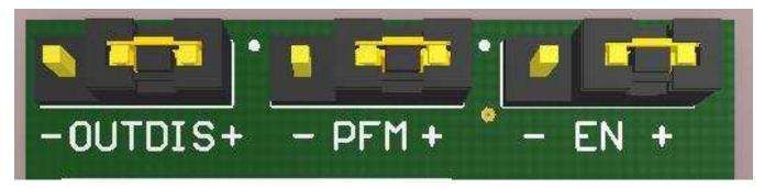
Figure 1. Enable Jumper Settings
