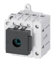
Load disconnector 3LD3, lu 32 A Main switch 3-pole + N Rated operating capacity for AC-23 A at 400V 11.5kW Installation in distribution boards, Basic switch without Knob-operated mechanism with auxiliary switch 1OE + 1S
