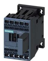
power contactor, AC-3 7 A, 3 kW / 400 V 1 NO, 24 V DC 0.85-1.85\* US, with varistor integrated, 3-pole, size S00, spring-type terminal not expandable with auxiliary switch
