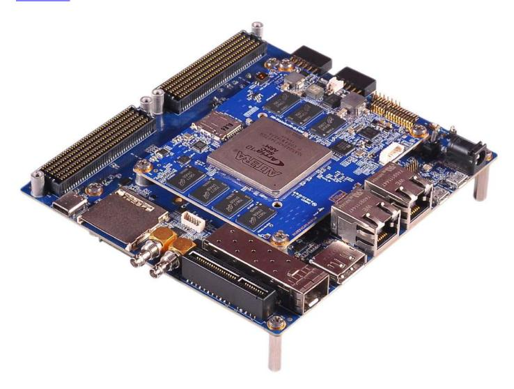
Figure 16: Arria10 SoC/FPGA SOM Development Platform
