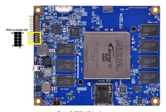
Figure 7: FPGA AS Header
