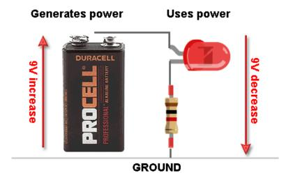
In our three-piece circuit, we have the battery (which generates voltage) and the resistor+LED (which uses up the voltage). I will now tell you a very key 'law' of electronics:
