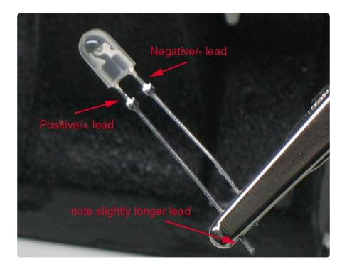
LEDs are so common, they come in dozens of different shapes and sizes. The LEDs you are most likely to use are the through hole LEDs with two legs. There are lots of LEDs that are small and hard to solder but these are easy to use with a breadboard because they have long wires we can stick in. The clear or clear-ish bulb is what protects the light emitter (thats where the magic happens). In fact, the first two letters of LED stand for Light Emitting.
