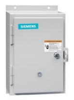
Reversing motor starter, Size 1, Three phase full voltage, Solid-state overload relay, OLR amp range 0.75-3.4A, 110V 50Hz / 120V 60Hz coil, Non-combination type, Enclosure type 12, Dust/drip proof for indoors, Standard width enclosure
