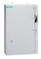
Non-reversing motor starter, Size 1, Three phase full voltage, Solid-state overload relay, OLR amp range 0.75-3.4A, 24VAC 50-60Hz coil, Combination type, 30A fusible disconnect, 30A/600V fuse clip, Enclosure NEMA type 4/12, Water/dust tight for outdoors, Extra-wide enclosure
