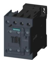
Contactor, AC-1, 50 A/400 V/40  $^\circ\text{C},$  S0, 4-pole, 220 V DC, 1 NO+1 NC, screw terminal
