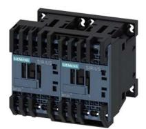
Reversing contactor assembly AC-3, 3 kW/400 V, 24 V DC 3-pole, Size S00 Spring-type terminal electrical and mechanical interlock with integrated diode
