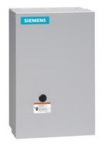
Mechanically held lighting contactor, Contactor amp rating 100A, 0 N.C. / 3 N.O. poles, 24VAC 60HZ coil, Non-combination type, Enclosure NEMA type 1, Indoor general purpose use
