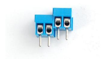
Find the terminal blocks, they're blue and come in 3-pin and 2-pin shapes. We'll need to slide the blocks together for the next step where we put the blocks into the proto plate. Slide them together to make 1x8 pin, 1x5 pin, and 3x4pin terminal blocks
