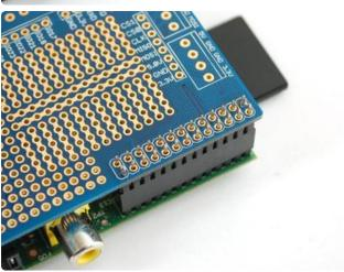
Heat up the soldering iron to 650 °F and wait for it to get up to temperature. Then heat a corner pad/pin with the iron tip and after two seconds poke in a small amount of solder. After the solder has melted into the pad/pin remove the iron.
