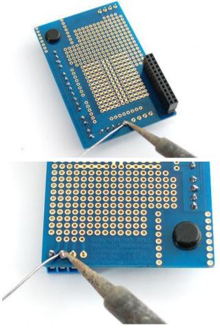
Solder each terminal block connection to the PCB using plenty of solder to make a strong mechanical connection
