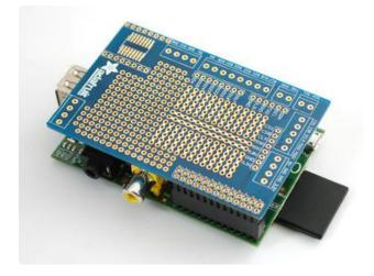
Place the proto plate PCB on so that the 2x13 header pins poke out through the matching 2x13 pads in the corner.
