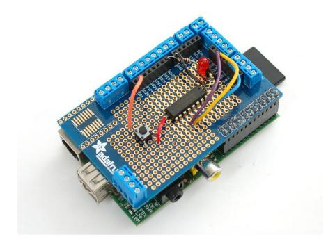
Now that you've finally got your hands on a Raspberry Pi® (), you're probably itching to make some fun embedded computer projects with it. What you need is an add on prototyping Pi Plate from Adafruit, which can snap onto the Pi main board assembly (and is removable later if you wish) and gives you all sorts of prototyping goodness to make building on top of the Pi super easy.
