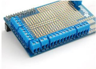
Place the blue terminal blocks around the perimeter of the Proto Plate PCB. Make sure you place them so that the open ends are facing out as shown.
