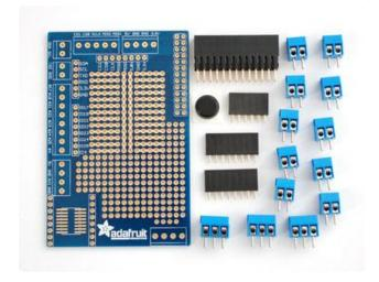
Check that you have all the parts - a PCB, a 2x13 female header, a 1x6 female header, two 1x8 female headers, bumper, three 3-pin terminal blocks and ten 2-pin terminal blocks
