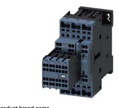
Contactor, AC-3, 15 kW / 400 V, 2 NO + 2 NC, 110 V AC, 50 Hz, 3-pole, Size S0 Spring-type terminal Removable auxiliary switch
