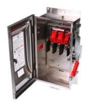
Siemens Low Voltage Circuit Protection Heavy Duty Safety Switch. 3-Pole 3-Wire Non-Fused in a type 4/4X 316 grade Stainless Steel enclosure. Rated 600VAC (60A).
