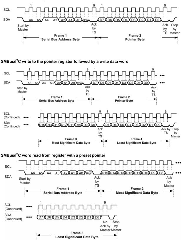
SMBus/I<sup>2</sup>C write to the pointer register
