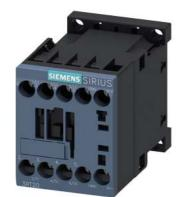
Power contactor, AC-3 7 A, 3 kW / 400 V 1 NO, 110 V DC 3-pole, Size S00 screw terminal
