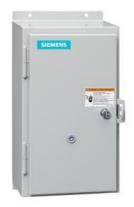
Non-reversing motor starter, Size 2 1/2, Single phase, 2-pole, Amb compensate bimetal OLrelay Contactor amp rating 60Amp 110V 50HZ / 120V 60HZ coil, Non-combination type, Enclosure type 12, Dust/drip proof for indoors
