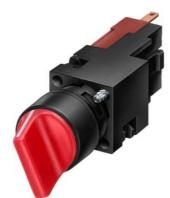
Selector switch, 16 mm, round, plastic, red, 3 switch positions I-O-II, latching, Actuating angle 2 x 62 degree, 1 NO, 1 NO  $\,$
