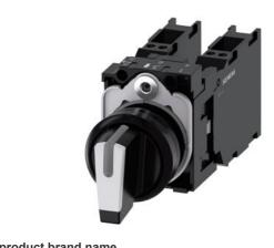
Selector switch, illuminable, 22 mm, round, plastic, white, selector switch, short, 3 switch positions I-O-II, latching, 10:30h/12h/13:30h, with holder, 2 x 1 NO+1 NC, spring-type terminal, with laser labeling, upper case and lower case, always upper case at the beginning of the word
