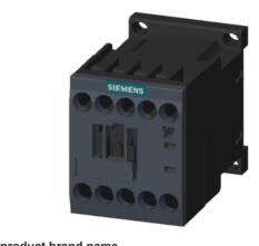
Power contactor, AC-3 12 A, 5.5 kW / 400 V 1 NC, 230 V AC, 50 / 60 Hz 3-pole, Size S00 screw terminal upright mounting position
