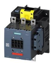
Power contactor, AC-3 150 A, 75 kW / 400 V Coil AC 50/60 Hz and DC 200-277 V x (0.8-1.1) F-SPS input 24 V DC 3-pole size S6 Auxiliary contacts 2 NO + 2 NC permanently mounted Main circuit: Busbar Control and auxiliary circuit: Screw terminal
