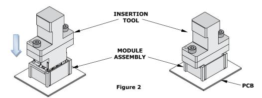
3. Using the insertion tool and an appropriate press, seat the header assembly until there is less than 0.10mm (.004") clearance between the bottom of the plastic housing and the surface of the PCB. See Figure 3.
