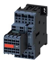
Power contactor, AC-3 38 A, 18.5 kW / 400 V 2 NO + 2 NC, 230 V AC 50/60 Hz, with inserted varistor 3-pole, Size S0 Spring type terminal Captive auxiliary switch
