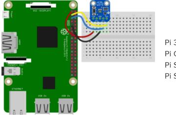
Pi 3V3 to sensor VIN Pi GND to sensor GND Pi SCL to sensor SCL Pi SDA to sensor SDA
