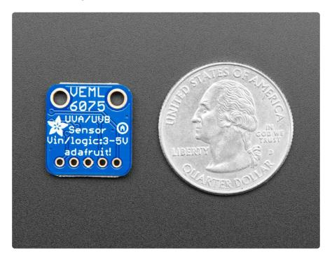
This UV sensor works great with 3 or 5V power or logic, its nice and compact, and its easy to use with any I2C-capable microcontroller. We have example code and libraries for Arduino () and CircuitPython/Python ().
