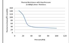
21-869 Gap Pad 1.0mm thick; 1 inch^2 test sample; Pressure step = 10psi
