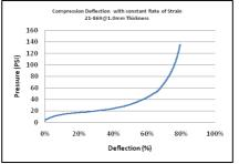
21-869 Gap Pad 1.0mm thick; 1 inch^2 test sample; Rate of strain = 1.0 mm/min
