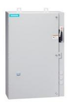
Reversing motor starter, Size 2, Three phase full voltage, Solid-state overload relay, OLR amp range 13-52A, Combination type, 60A disconnect switch, Encl NEMA type 4X 304 S-Steel, Water/dust tight noncorrosive
