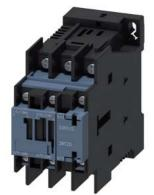
power contactor, AC-3 9 A, 4 kW / 400 V 1 NO + 1 NC, 24 V DC 3-pole, Size S0 ring cable lug connection
