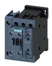
Contactor, AC-1, 35 A/400 V/40  $^{\circ}$ C, S0, 4-pole, 110 V AC/50 Hz, 120 V/60 Hz, 1 NO+1 NC, screw terminal
