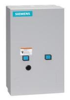
2-speed 3-phase motor starter, Size 1, Two separate windings, Constant or variable torque, Solid-state overload relays, Low Spd OLR range 0.75-3.4A, High Spd OLR range 0.75-3.4A, 24VAC 50-60Hz coil, Enclosure NEMA type 1, Indoor general purpose use
