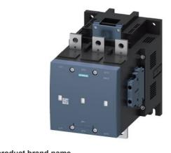
vacuum contactor, AC-3 400 A, 200 kW / 400 V AC (50-60 Hz) / DC operation 240-277 V AC/DC auxiliary contacts 2 NO + 2 NC 3-pole, frame size S12 busbar connections drive: conventional
