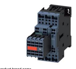
Contactor, AC-3, 15 kW / 400 V, 2 NO + 2 NC, 110 V AC, 50 Hz, 120 V, 60 Hz, 3-pole, Size S0, Spring type terminal Captive auxiliary switch
