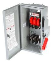
Siemens Low Voltage Circuit Protection Heavy Duty Safety Switches. Type: ENCLOSED, SAFETY SWITCH Std: CSA V. Rating: 600V A. Rating: 30 A Wattage: 3W No. Of Poles: 3P F. Rating: 60Hz Action: SINGLE THROW Material: 304SS Enclosure: TYPE 3R. 2-3 point mounting holes. O. Cycles: 10000 O. Temperature: (-20F-120F) AMBIENT TEMPERATURE Environmental Conditions: OUTDOOR
